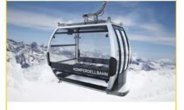
Numbers / Dates / Facts: Bottom station: 1,442 m Mid station: 1,610 m Top station: 1,982 m Length of 1st section: 566 m Length of 2nd section: 2,075 m Total length: 2,641 m Altitude difference: 540 m Transport capacity: 3,000 persons/hour (3,500 persons/h in the final stage) Number of supports: 20 supports Travel time: 10.5 minutes Construction costs: 50 million euros
